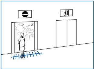
The event is triggered when the specified number of objects have crossed the directional beam that is configured over the camera's field of view in the selected time period. The beam can be unidirectional or bidirectional.
