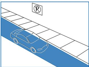
The event is triggered for each object in a region of interest that stops moving for the specified threshold time.
