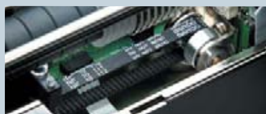
High-durability Synchro Belt Drive and HB Stepper Motor
