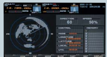
•Antenna Bearing Indication using Great Circle Map
