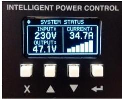
Figure 9: ICM Front Control Interface – System Status Screen
