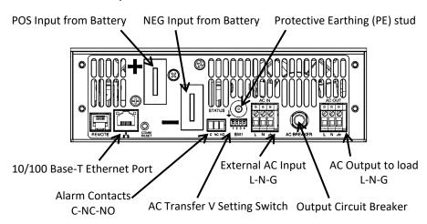
Figure 4: Back Panel Connections
