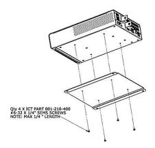
Figure 2: Inverter Wall Bracket Mounting
