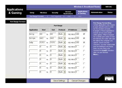
Figure 13: Typical Router Port Forwarding Screen
