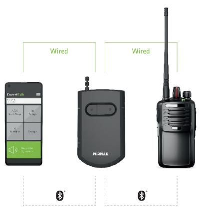
Roger Covert C can handle one Bluetooth® link while Roger Covert Dual C separable radio can handle simultaneously one Bluetooth® link and one wired link.
