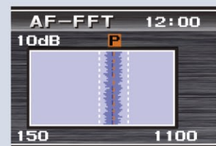
AF-FFT scope (waterfall display)
